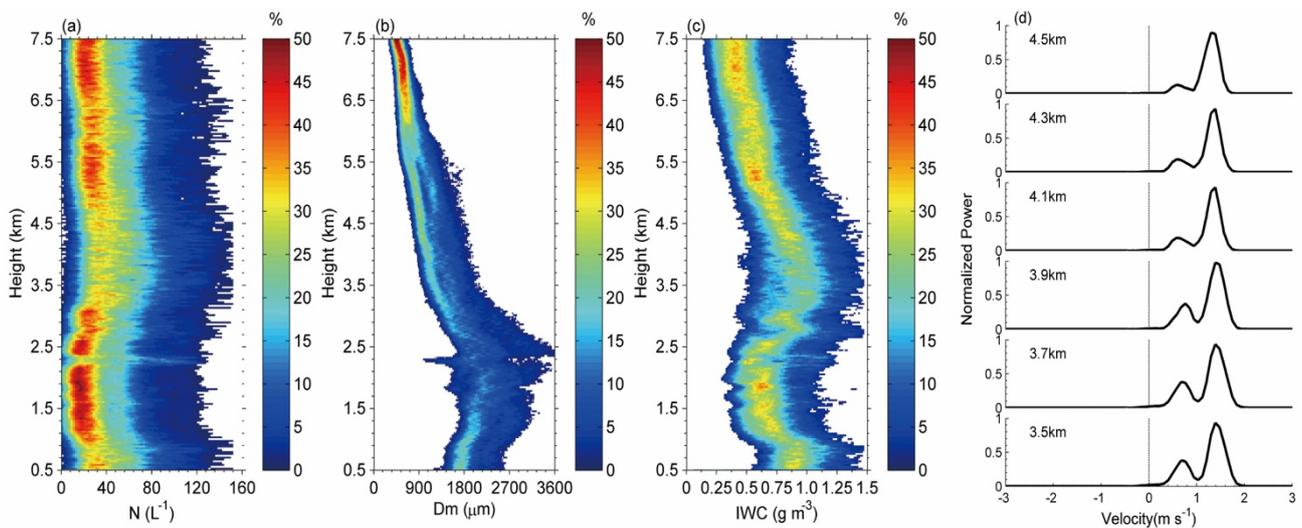
Figure 1. The CFADs of (a)  $N$ , (b)  $D_m$ , and (c) IWC in the St region during 0020 to 0120 UTC on 28 Feb 2015; and (d) is the diagram of normalized bimodal spectra between 3.5 and 4.5 km. The resolutions of CFADs are 20, 100, and 0.1 respectively for  $N$ ,  $D_m$ , and IWC.
