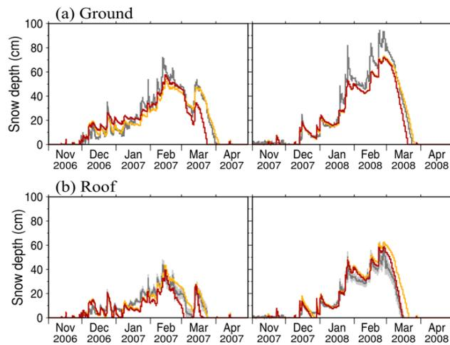
Figure 1. Seasonal variation in snow depth (a) on the ground around a building and (b) on the roof during two winters. Gray, yellow and red lines represent the observations, and our offline simulations using sSPUCdgn and sSPUCprg, respectively.
